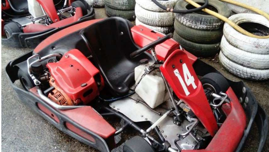
Photograph 4.3: Sodikart gas-powered 270 cc kart.
